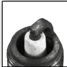
Spark plug has dry deposits
